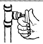
2) Turn "OFF" the water to the water heater. Some installations require that the water be turned off to the entire house.
